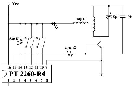
UHF Band 4-Data Transmitter Circuit is recommended.
